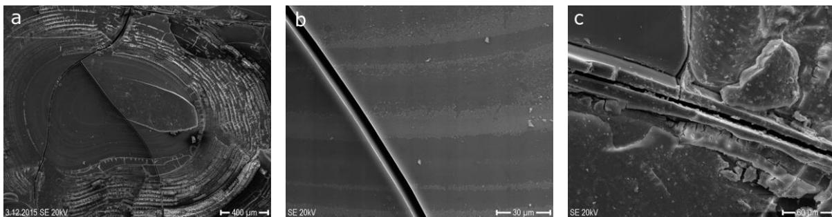
Figure 1: Sample FN1369\_Ob62; SEM- examination of gel layer, which has separated as a compact lamellar network from the glass matrix. a) inner areas of gel layer, originally connected to the glass matrix; b) cracks forming independently from lamellar network; c) cracks at the border zone of lamellar networks, which also show different structural directions.
