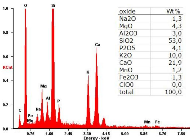
Figure 2: EDX-spectrum of sample FN933\_Ob65 showing the glass composition (Average of three-point measurement within the glass matrix). Despite an intensive blue coloration of the sample, no additives were detected.
