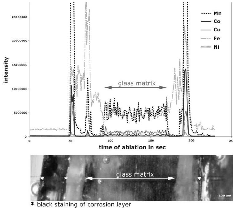
Figure 3: Sample FN933\_Ob66; Intensity profile of laser ablation line-scans applied on a cross-section of the glass sample. While the scan detected accumulation of coloration elements Co, Ni, Cu, and Zn in those areas of the gel layer, which show black staining by manganese enrichment, the light areas of the gel layer were analysed with a lack of coloring elements.
